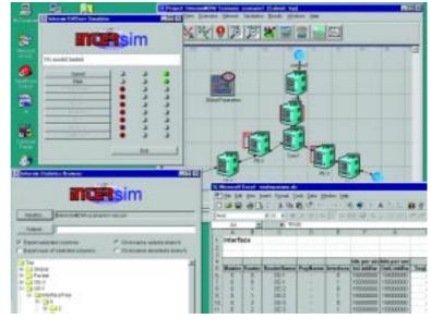
EPCC has completed the world's first packet-level simulation tool for differentiated service networks. Intersim is a tool that simulates Cisco equipment for IP quality of service on diffserv networks, to help designers build better networks.
