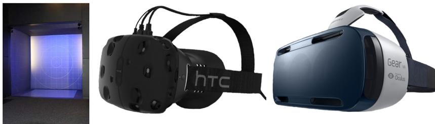
**Fig. 1.** CAVE-like system (left), HTC Vive (center) and Samsung GearVR (right)
