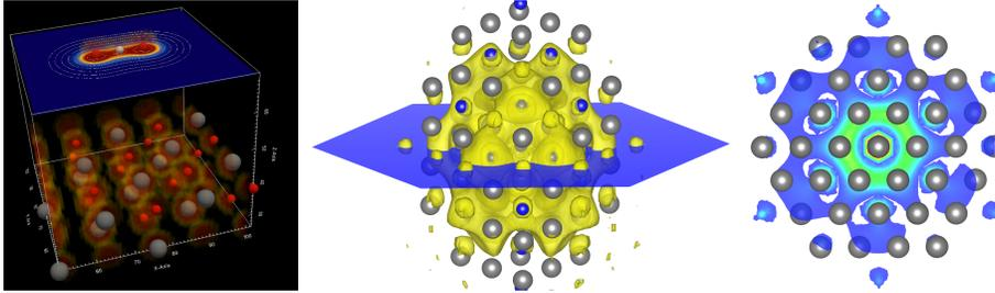
**Fig. 2.** Adsorption of  $\text{CO}_2$  on  $\text{CaO}(001)$  surface, using the Paraview software [1] (left), and exciton in LiF, shown in 3D (center) or 2D (right), using the Vesta software [12]
