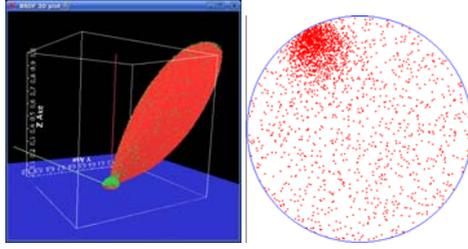
**Fig. 1.** Both images show a distribution of 2500 samples obtained with our disc method. The left one shows how the samples match the BRDF function (in red). The image on the right is the projection on disc of those directions.
